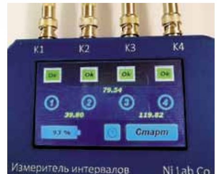
Fig. 4. The VoD-305 measuring instrument (Australia) – а; the IVI-4 microsecond time interval meter (Design and Engineering Bureau “INTERVAL”, Novosibirsk) – б
